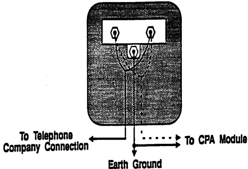
2. Connect one end of the 12 AWG earth ground wire to the center terminal on the TII Protector.
