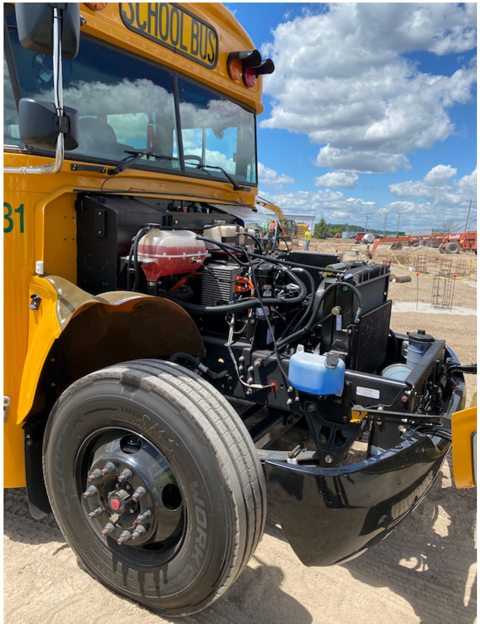
Beneath the electric bus to be used by Lake Shore Central School District are 14 batteries. The open hood exposes an area that would house a 1,500-lb. engine in a traditional diesel-powered bus.
